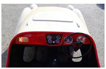
Alan is a real detail man, and this shows through on the restoration, an example being the dashboard gauges. Where original gauge bezels were missing, Alan recreated these on his lathe, and where original
