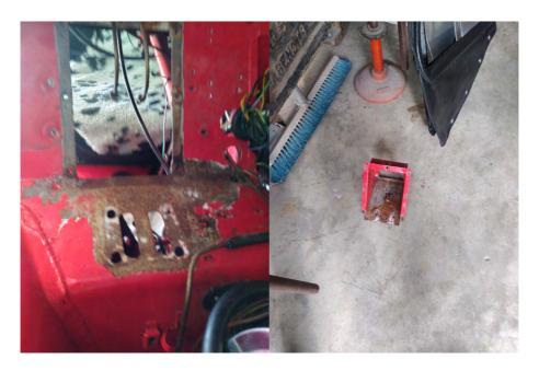
For us this has been attending to the mess that brake fluid made to the bulkhead. Brake fluid certainly makes a good paint stripper. While at the panel beaters a small rust patch in the door was attended to. Some other areas taken care of as well. Warren had an issue with the A pillar of his TR2 which needed welding. His TR8 however is going well - the issues encountered at this year's Nationals now resolved.
